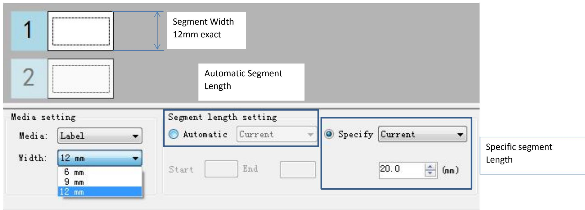
**Automatic segment length** will adjust the segment length according to the inputting content, min. 6mm upto max. 100mm
